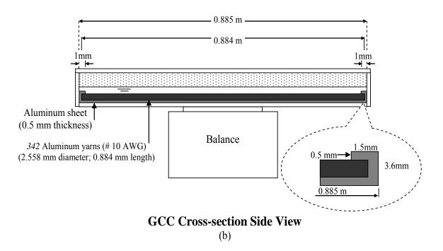
Fig. A16 – A GCC using distilled Water.
