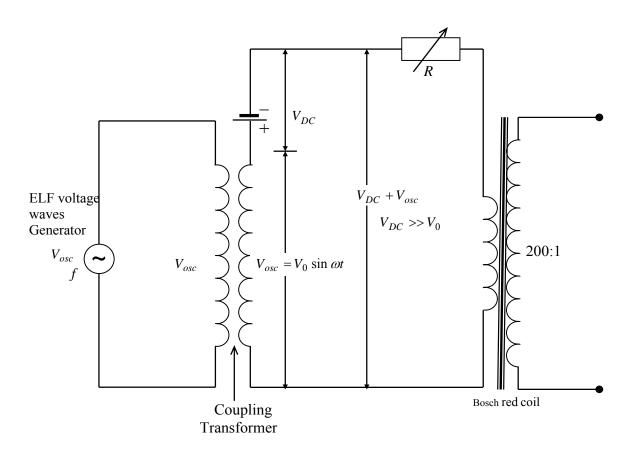
Fig. B3 – Equivalent Electric Circuit
